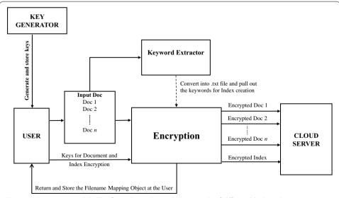
**Figure 3** Encryption module. The *figure* shows the working principle of different blocks in the encryption module of the PrivCloud system. The encryption module provides the document and index encryption functionality.
