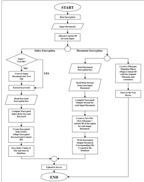
**Figure 6** Flowchart for the document and index encryption process. The *figure* shows the flowchart of the encryption module for the PrivCloud system. It provides detail work-flow of the module to compute the encrypted document and encrypted index.
