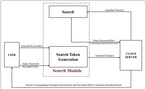
**Figure 4** Search module. The *figure* shows the working principle of different blocks in the search module of the PrivCloud system. This module enables a cloud user to generate an encrypted query to the server. The cloud server can use this encrypted query to search over the encrypted data without knowing the contents of the data or the query.
