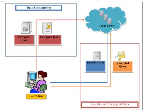
**Figure 2** Working principle of adaptively secure SSE scheme to search over encrypted data. The *figure* shows the work-flow of the searchable symmetric encryption scheme. This scheme generates and stores an encrypted index at the cloud server to enable search over encrypted data.
