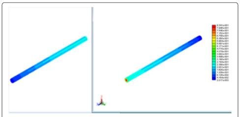
Figure 5 Current distribution of arm 1 and arm 2 in dipole antenna [current is higher near the feeding point and becomes zero and start its path as a electromagnetic wave for communication at rear end].
