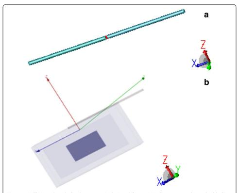
Figure 1 Half- Wave length dipole antenna is designed for 900MHz frequency and is embedded in Mobile phone casing for Near field interaction analysis. a Dipole Antenna [simulated dipole antenna with excitaion feed at the centre]. b Mobile Phone Model [mobile handset model with dipole antenna embedded].
