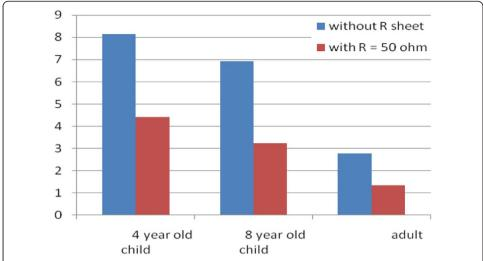
Figure 11 Graphical representations of 10 g – SAR values for children and adult [analysis indicates that resistive sheet in mobile phone handset considerably reduces the power coupled to human head].
