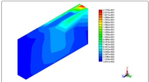
Figure 3 Current distribution in mobile phone [currrent is more near the antenna excitation feed shown by red colour in the simulation result].
