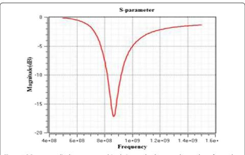
**Figure 6** S-Parameters dipole antenna port [simulation results shows good return loss of more than 15 dB, suitable for mobile communication].
