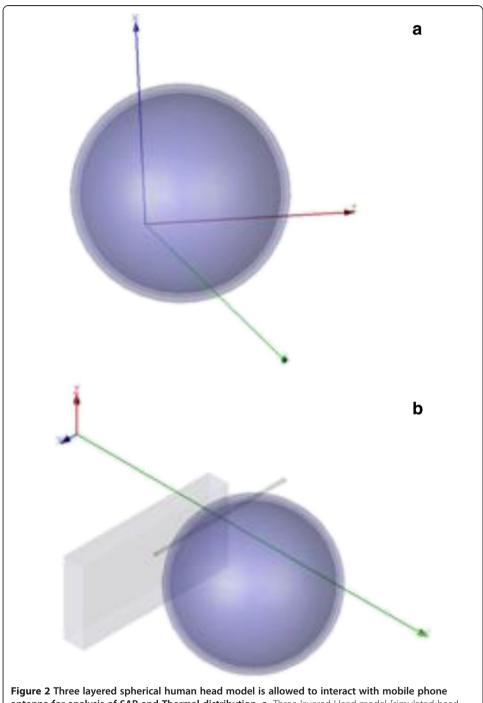
**Figure 2** Three layered spherical human head model is allowed to interact with mobile phone antenna for analysis of SAR and Thermal distribution. **a.** Three layered Head model [simulated head model with skin, skull and brain layer]. **b** Mobile phone interaction with head [mobile phone handset interacted with three layered head model].
