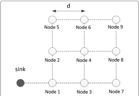
**Figure 12 Network topology used.** The dark node is the sink node while the blank nodes are the video node. Each node is given an identification number according to its distance to the sink. Therefore, node1 is closer to the sink than node2, and so on. Each video node located at a specific location in the topology illustrated in this is attached to the camera located at the same location shown in Figure 1.
