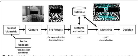
**Fig. 3** Biometric Recognition process in the evaluation. Examples of the images obtained are over the Capture and Pre-process boxes. Over the Matching box is an example of the SIFT application.
