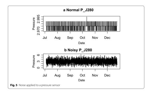
sensor reading between October and November. These readings are from the first attack dataset and that spike corresponds to an attack that eventually led to an overflow of Tank 1. Looking at the noise readings it can be seen that the spike is no longer visible thus making it more challenging to detect that attack.
