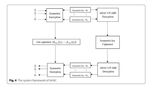
keys. It is clear from our framework that only one encryption and decryption operation is needed to share multiple files securely, while traditional schemes have to do multiple encryption and decryption operations.
