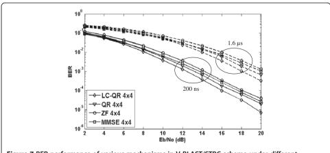
Figure 7 BER performance of various mechanisms in V-BLAST/STBC scheme under different maximum delay spread environment.
