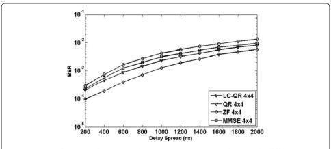
Figure 8 BER performance of various mechanisms in V-BLAST/STBC scheme under different maximum delay spread environment at 16 dB.
