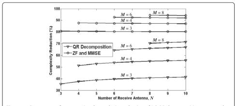
Figure 11 Percentage of computational complexity reduction of LC-QR decomposition compared to ZF, MMSE and QR decomposition with different M and N for  $N \ge M$ .
