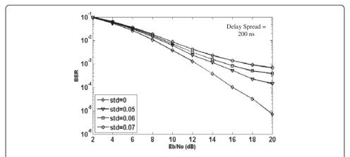
**Figure 9** BER performance of LC-QR  $4 \times 4$  with different standard deviations of channel estimation error  $\sigma_E$  and delay spread = 200 ns.
