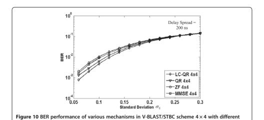
standard deviations of channel estimation error  $\sigma_E$  and delay spread = 200 ms at 16 dB.
