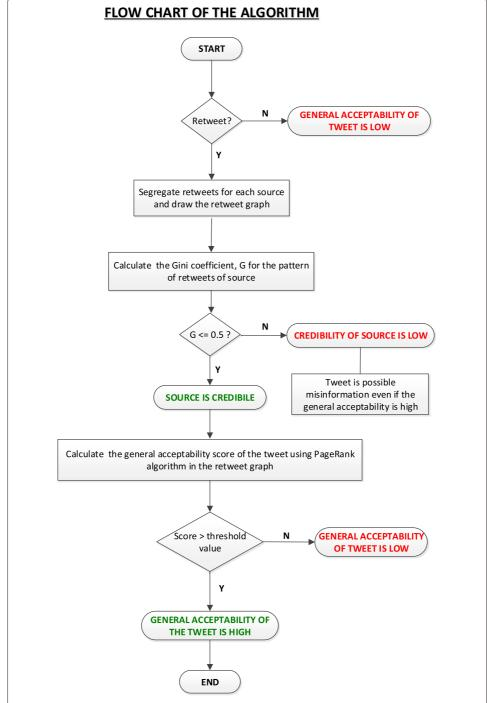
**Figure 6 Algorithm for determination of misinformation in tweets.** The flowchart giving the algorithm to detect misinformation using a retweet graph to estimate the general acceptability of tweets and credibility of sources.
