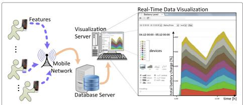
**Figure 2 CoenoFire: smartphone based data collection framework.** Raw smartphone sensor data is saved to the SD-Card and features are transmitted via the mobile network to enable real-time monitoring of performance metrics and system status, e.g. battery level.
