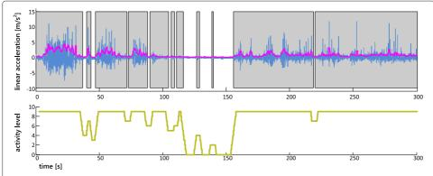
**Figure 5 Calculation of activity level.** Top: Linear acceleration magnitude and moving standard deviation (pink), rectangles indicate segments in which the standard deviation exceeds the activity detection threshold. Bottom: Activity level calculated on a hopping window ( $L=5 \, \text{s}$ ,  $S=200 \, \text{ms}$ ).
