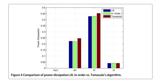
2% higher than that of the LR algorithm. In terms of overall power-performance benefits, our proposed LR algorithm outperforms the Tomasulo algorithm. In our experiment, it was also observed that the fraction of clock power dissipation is almost the same for both algorithms. This significant increase of clock power in Sim-Panalyzer is mostly due to the fact that it is dependent on the dynamic power consumption.
