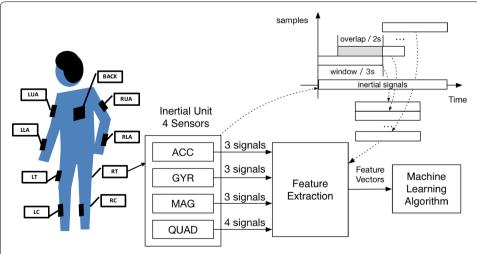
**Fig. 1** System architecture (the sensor placement is referenced from [24]). The system architecture includes two steps: feature extraction and activity classification. This system includes 9 inertial measurement units generating and every unit contains four sensors, accelerometer (ACC), gyroscope (GYR), magnetometer (MAG) and quaternion (QUAD) sensor
