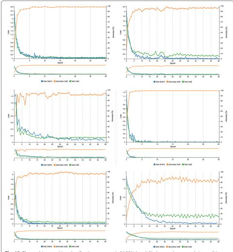
**Fig. 12** The washing machine classification accuracy is 96.85% (*top-left*); the stand-mounted air-conditioner accuracy is 96.85% (*top-right*). The centerlines are arranged in the order of wall-mounted air-conditioners (93.75%), robotic vacuum cleaners (99.9%). The *lines* at the *bottom* are arranged in order of vacuum cleaners (96.1%) and microwaves (85.9%), for all of which we extract only the object area and use the image for classification
