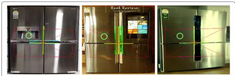
**Fig. 9** Extract center point using *horizontal* and *vertical edges* of the center, and then extract Sobel-filtered image from perspective-warped image
