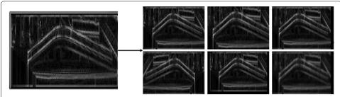
**Fig. 8** Extract a Sobel filtered image and convert it into six distorted (resize, move a few pixels to the left and right, and we flip left and right for each images) images for using classification
