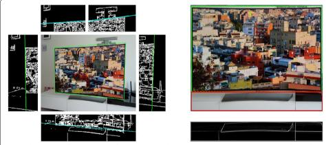
**Fig. 2** The process of pre-processing for recognizing Television; extract 4 vertices using 5 edges (divide the *upper edge* into two parts to account for the curved display), extract lower end from a warped perspective image and extract a Sobel filtered image
