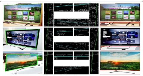
Fig. 7 Extract 4 vertices using 5 edges, extract lower end from a warped perspective image
