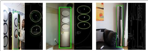
**Fig. 4** The process of extracting additional information for recognizing the stand-mounted air conditioner: find fit circles from a canny edge and cluster them. Circular wind holes are arranged from one to three based on size. The fact that the wind hole is not circular also affects the final outcome
