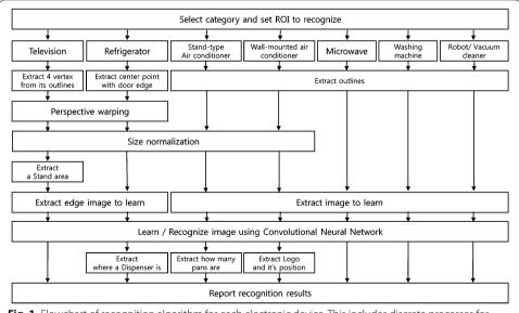
**Fig. 1** Flowchart of recognition algorithm for each electronic device. This includes discrete processes for extracting features to normalize and recognize images
