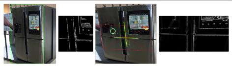
**Fig. 3** The process of pre-processing for recognizing a refrigerator: extract center point using *horizontal* and *vertical edges* of the center, and then extract Sobel-filtered image from perspective-warped image
