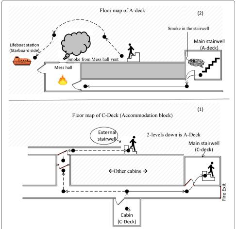
**Fig. 3** Floor map for decks A and C in AVERT simulator. A participant starts from Cabin (S) in part (1) and ends either at the mess hall or the lifeboat station in part (2) using external stairwell or main stairwell. The dotted lines show the alternate route, and the solid lines refer to the primary route
